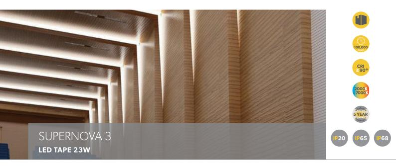
Supernova 3 is a superior quality commercial grade 24V 23W/m CRI 90+ LED strip with an output of 2054 lumens per metre for 3000K, 2185 lumens per metre for 4000K and 2300 lumens per metre for 6000K in IP20. Dimmable with the correct control gear options.
