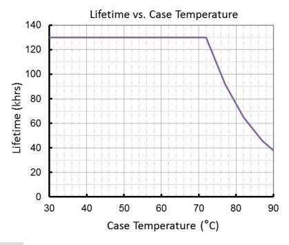
End of Life: Maximum Failure Rate = 10%
